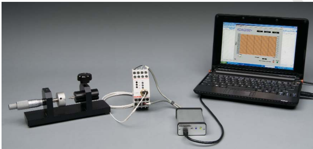
Typical system setup includes the KDAQ200+, Kaman KD-2306 sensor and electronics, PC, and appropriate USB cabling.
