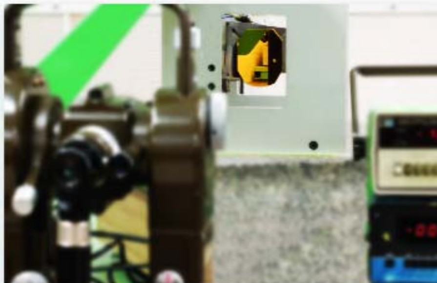
Theodolite incident angle measurement for optical assembly linearization calibration
