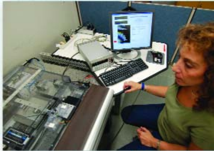
Automated laser interferometer calibration
