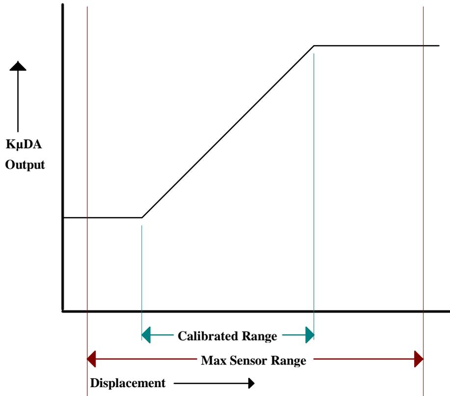
Figure 5: Displacement Output Voltage vs. Calibration Range
